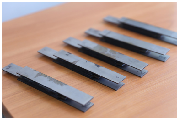
Sample of a new viscoelastic material connecting surfaces
